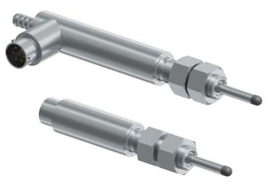
The HGSI GH-750-A series AC Spring Loaded Linear Variable Differential Transformer (LVDT) Position Sensors are used to monitor and track the linear motion or position of a target. These spring-loaded ruggedized sensors are ideal for use in industrial and laboratory applications including automotive R&D, motorsports, industrial, motion control, medical, military and aerospace.
