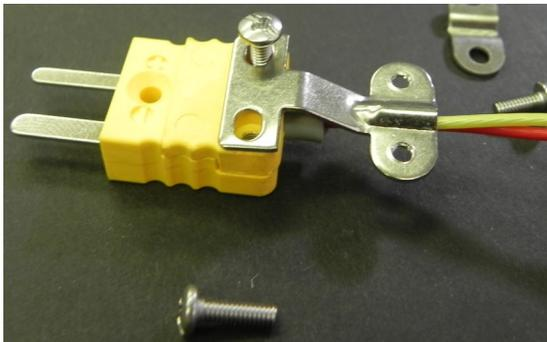
Replace cover, place strain relief on top of cover, and secure using long pair of screws.
