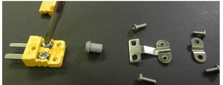
Loosen screw terminals that hold wire in place.
