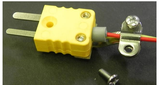
Flip connector over and using short screws, tighten small clamp, securing both wires. Complete!
