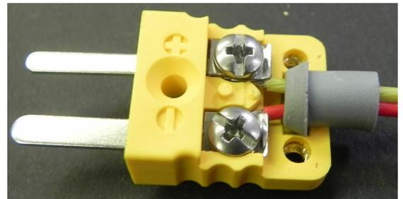
Secure wires under screw terminals.
